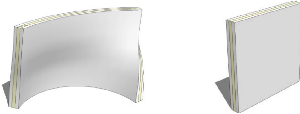
Figure 1.7 – Freeform to-be-printed wall (left) and simplified printed shear wall as studied in this thesis (right)
