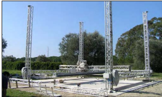
Figure A.16 – 5 x 5 x 5 m D-Shape printer (Krassenstein, 2014)
